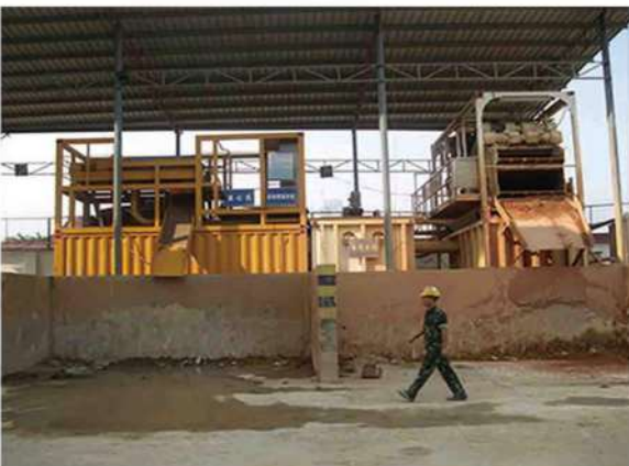
Shield mud-water separation system
