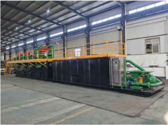
Refining sludge treatment system
